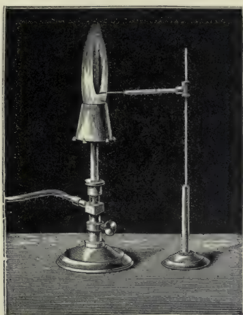
FIG. 182.—Coloured Flame of Salts in the flame of a Bunsen's Burner.
